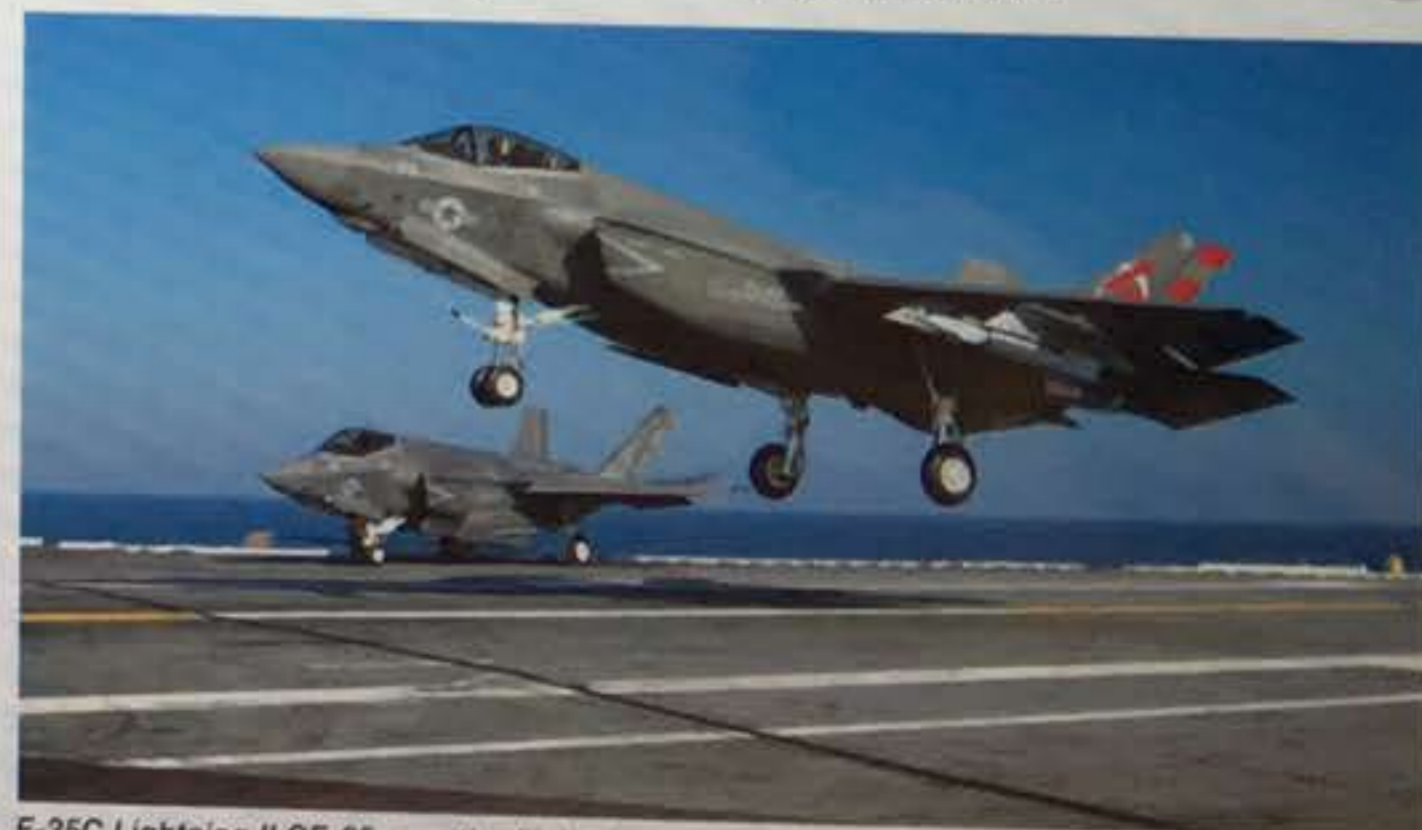
F-35C Lightning II CF-05 over the flight deck of the USS George Washington immediately before catching the wire. The aircraft is loaded with one inert GBU-12 laser-guided bomb. Michael Jackson/Lockheed Martin
