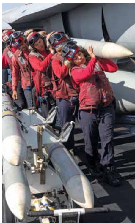
Below: This is how the armourers remove or attach weapons on the flightdeck.
