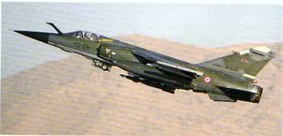
An F1CR 647/112-CB departs Kandahar airport for a close-air support mission. Mounted under the centerline station is a Paveway IV laser-guided bomb. (ETZEL DE VRIES)
