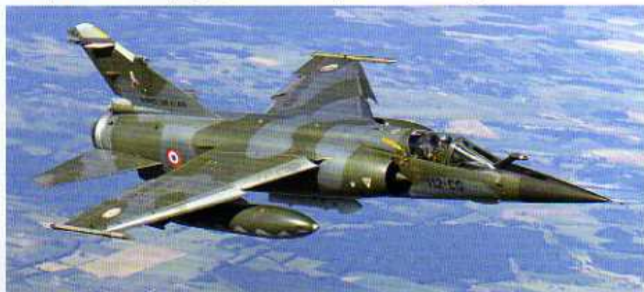
Like most aircraft of its generation, the Mirage F1 is of all-metal construction, with no significant use of advanced alloys or composites. The fuselage is of a conventional semi-monocoque construction. The wings have two main spars and four auxiliary spars.
