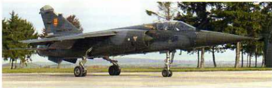
Above: In a clean configuration, devoid of pylons and stores, the Mirage F1 is one of the sleekest looking aircraft currently flying. This F1CT 236/ '30-QR' pauses for the camera prior to taxiing out for a training sortie.
